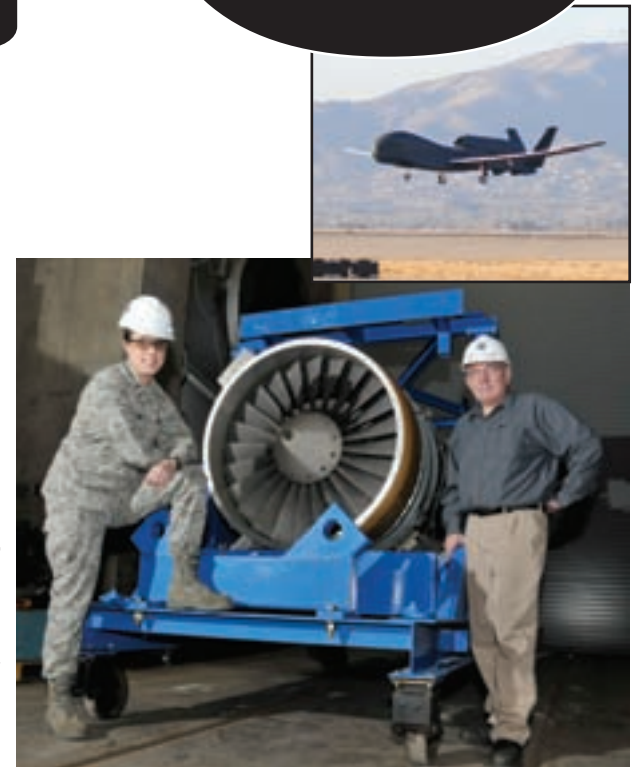
The Rolls-Royce AE3007H growth engine, which is the power plant for the RQ-4 Global Hawk unmanned aircraft system, underwent altitude testing at AEDC's T-4 test cell. The engine has upgraded turbine hardware and an improved combustor that are aimed at enabling the engine to have greater service life.
