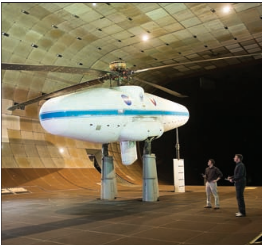
A full-size UH-60A Blackhawk helicopter rotor was the subject of tests conducted by NASA's Subsonic Rotary Wing Project. NASA collaborated with the U.S. Army and the U.S. Air Force at the National Full-Scale Aerodynamics Facility at NASA's Ames Research Center in Moffett Field, California. The test series that started in January and ended in May was designed to gather data on the rotor blades and air movement that the blades create in hopes of making new designs quieter, faster and more fuel efficient.
