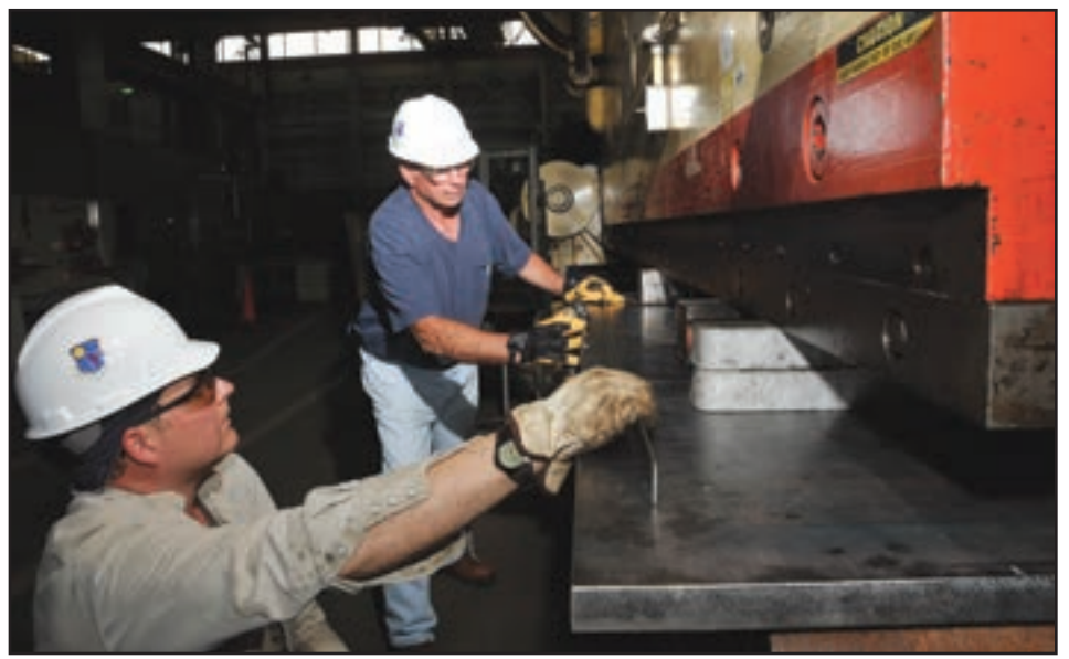
Above, Tim Taylor and “Chief Craftsman” Rodger Ford, ATA boilermakers, operate the 500-ton press brake to straighten the vertical housing front cover for the 4T CTS, before the part is heat treated. Below, ATA boilermaker Rusty Hargis works on the 4T CTS Doghouse. (Photos by Rick Goodfriend)
