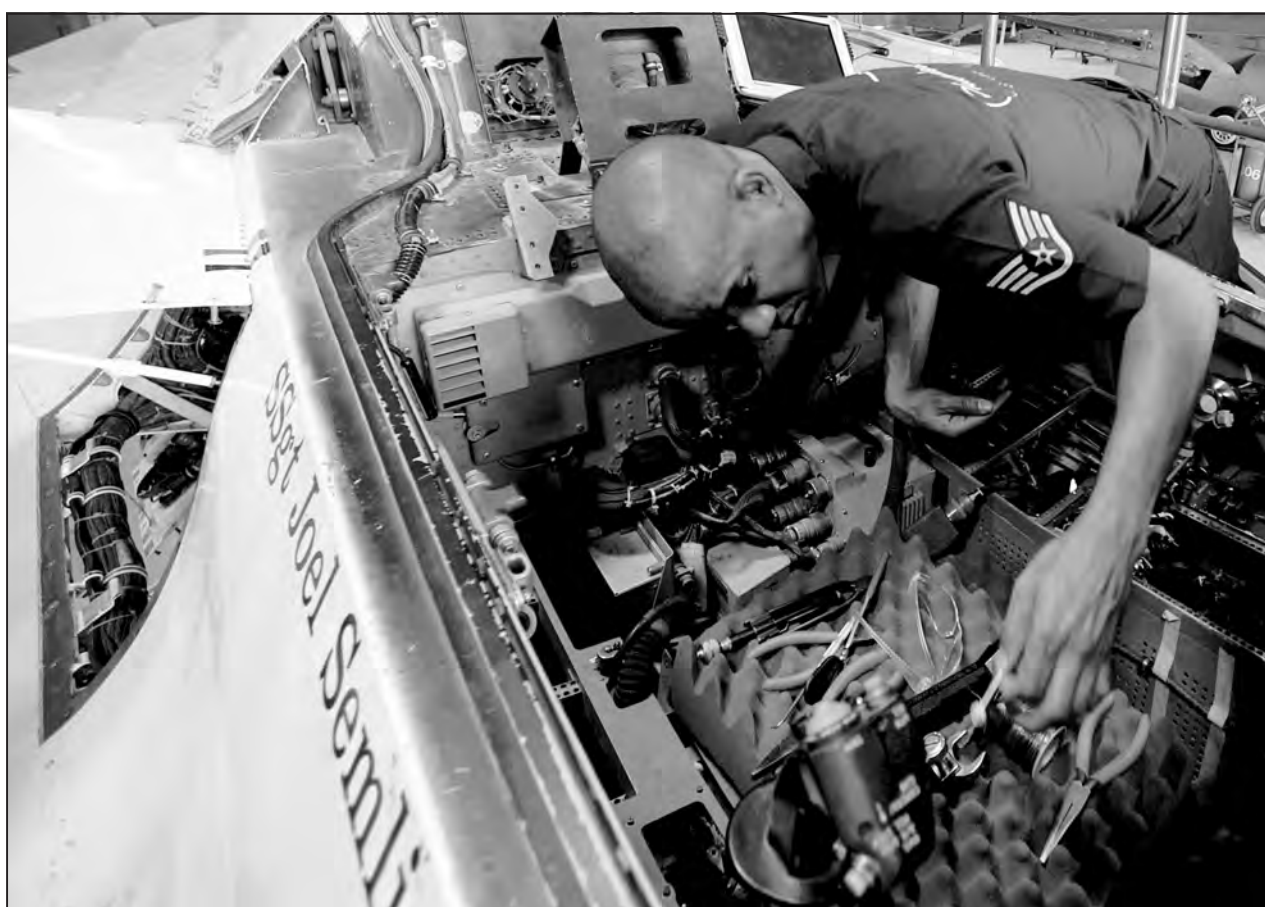
Staff Sgt. McGarry Lansiquot grabs a tool to repair internal parts of a Thunderbird F-16 Fighting Falcon's egress seat system at Nellis Air Force Base, Nev., May 20. (U.S. Air Force photo/Staff Sgt. Larry E. Reid Jr.)
