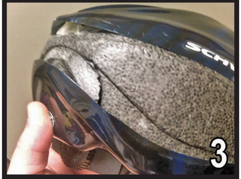
Figure 1: Top view of bicycle helmet – no apparent damage. Figure 2: Aft interior of bicycle helmet shows cracked foam insulation where impact to head occurred. Figure 3: Aft exterior of bicycle helmet shows cracked foam insulation and damaged plastic where impact to head occurred. (Photos provided)
