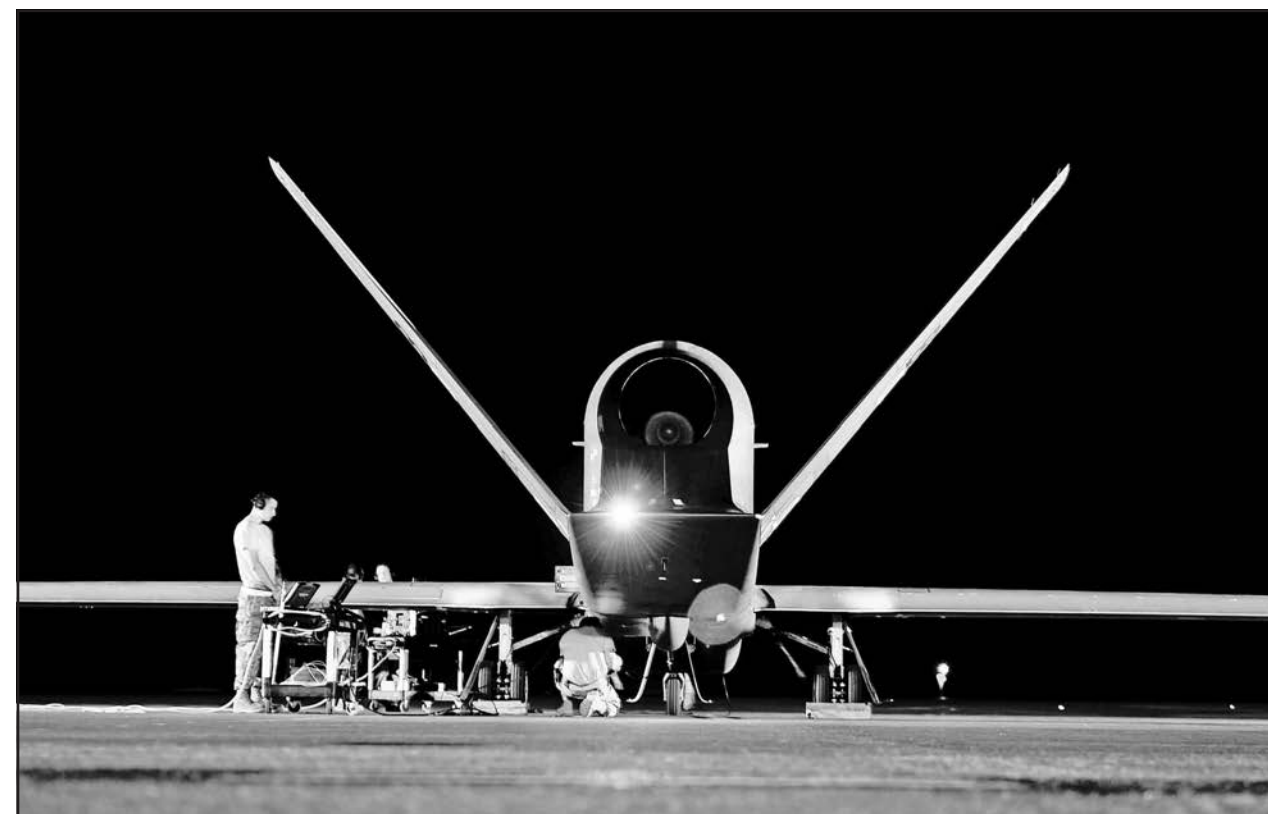
An RQ-4 Global Hawk undergoes pre-flight checks from maintenance technicians before a mission while deployed at an air base in Southwest Asia. Equipped on a block 40 Global Hawk, the Air Force completed the first Maritime Modes program risk reduction flight. The system is designed to provide intelligence, surveillance and reconnaissance information on vessels traveling on the water's surface. (U.S. Air Force photo/Staff Sgt. Andy M. Kin)
