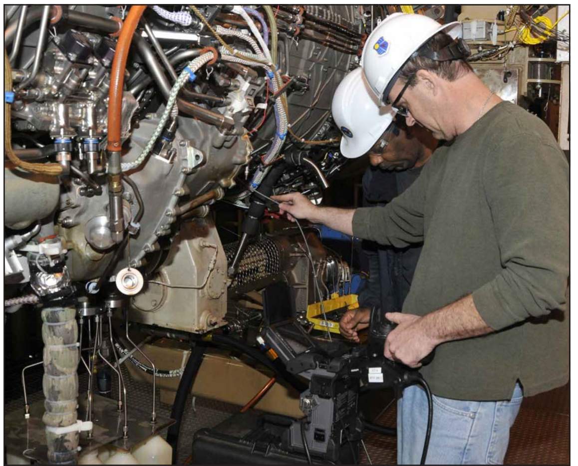
ATA Test Engineer Darren Carroll, pictured in front, assists as Pratt & Whitney Test Engineer Ronnie Thomas does a borescope inspection of the fan on the F135 engine. (Photo by Jacqueline Cowan)
