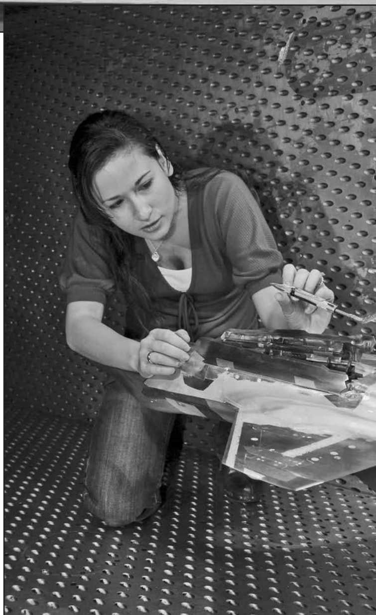
Monique Purdon, Lockheed Martin's wind-tunnel lead on the F-35 Lightning II store separation team, examines a GBU-39 Small Diameter Bomb (SDB) in the AEDC four-foot transonic wind tunnel. (Photos by Rick Goodfriend)
