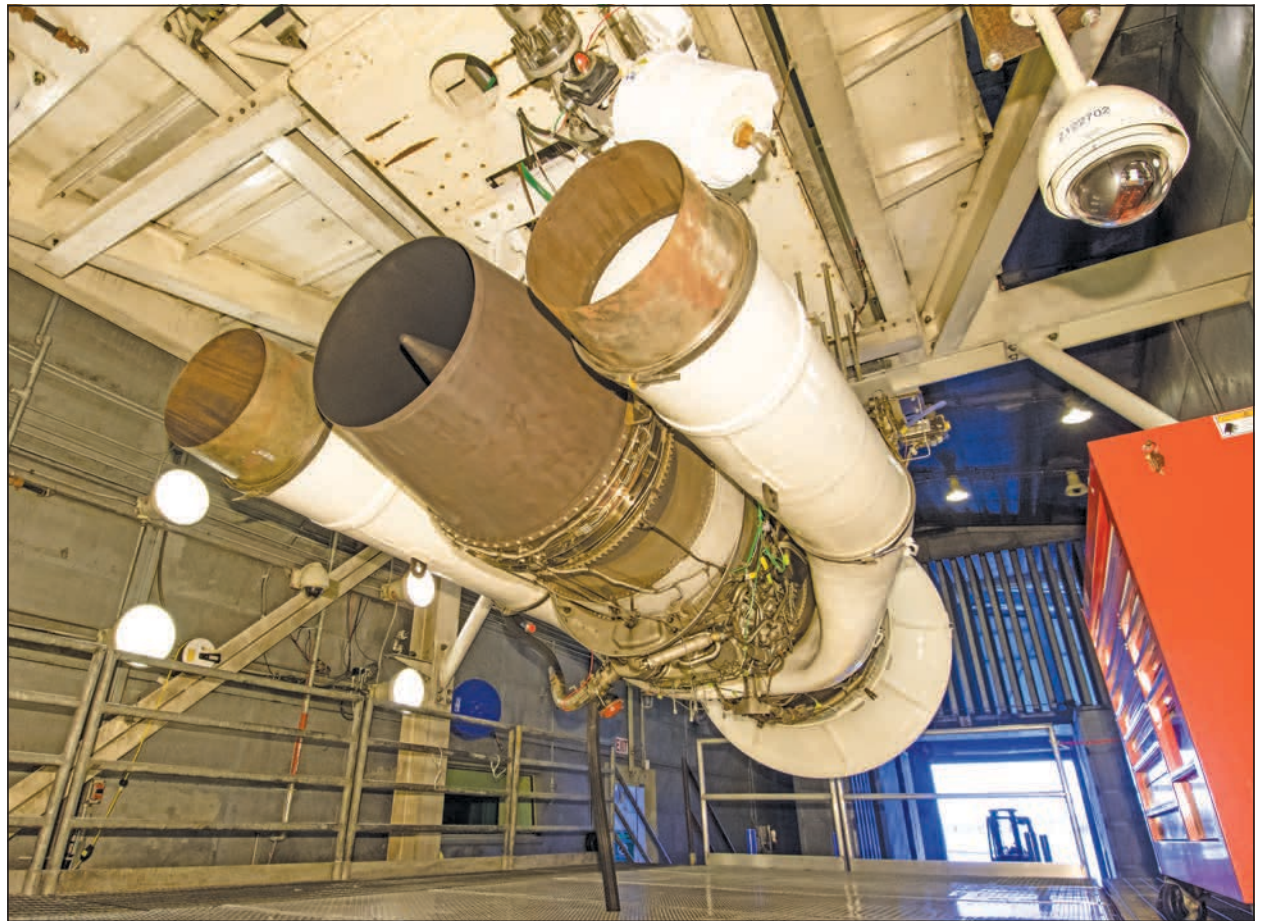
The TF33 Pratt & Whitney engine undergoes testing in an AEDC sea level test cell, to verify and validate newly redesigned components of the engine. The TF33 has powered several different military airframes, including the Boeing KC-135 Stratotanker, E-3 Sentry Airborne Warning and Control System and the E-8 Joint Surveillance Target Attack Radar System. (U.S. Air Force photo/Rick Goodfriend)
