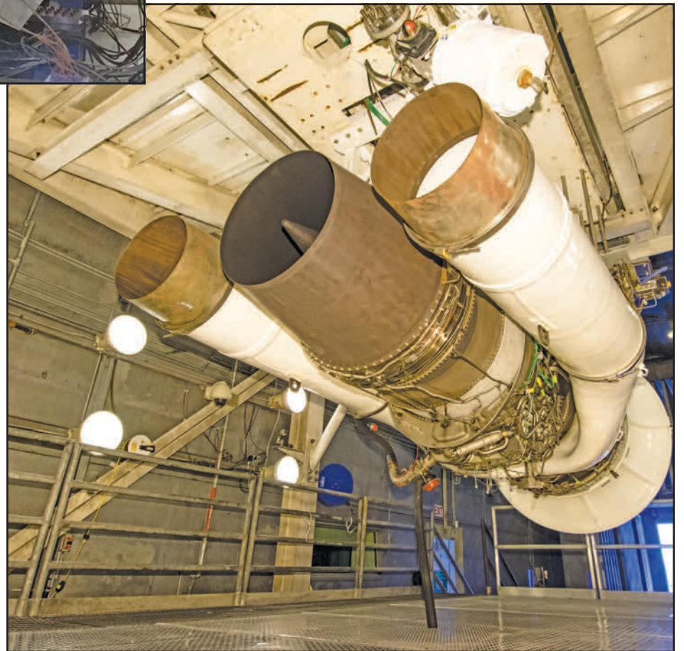
The TF33 Pratt & Whitney engine underwent testing in an AEDC sea level test cell, to verify and validate newly redesigned components of the engine. The TF33 has powered several different military airframes, including the Boeing KC-135 Stratotanker, E-3 Sentry Airborne Warning and Control System and the E-8 Joint Surveillance Target Attack Radar System. (U.S. Air Force photo/Rick Goodfriend)
