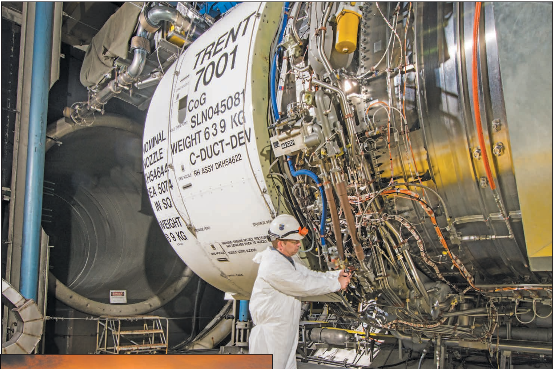
Dan Haden, lead outside machinist at AEDC, helps prep the Rolls-Royce Trent 7000 engine for testing in the C-2 engine test cell. The engine will be used in the new Airbus A33neo. Jit Sahota, engine management engineer for Rolls-Royce Trent 1000 and 7000 projects, said testing at AEDC was conducted to affirm the combined capabilities that Roll-Royce was striving for in this engine and it was achieved. (U.S. Air Force Photo/Jacqueline Cowan)
