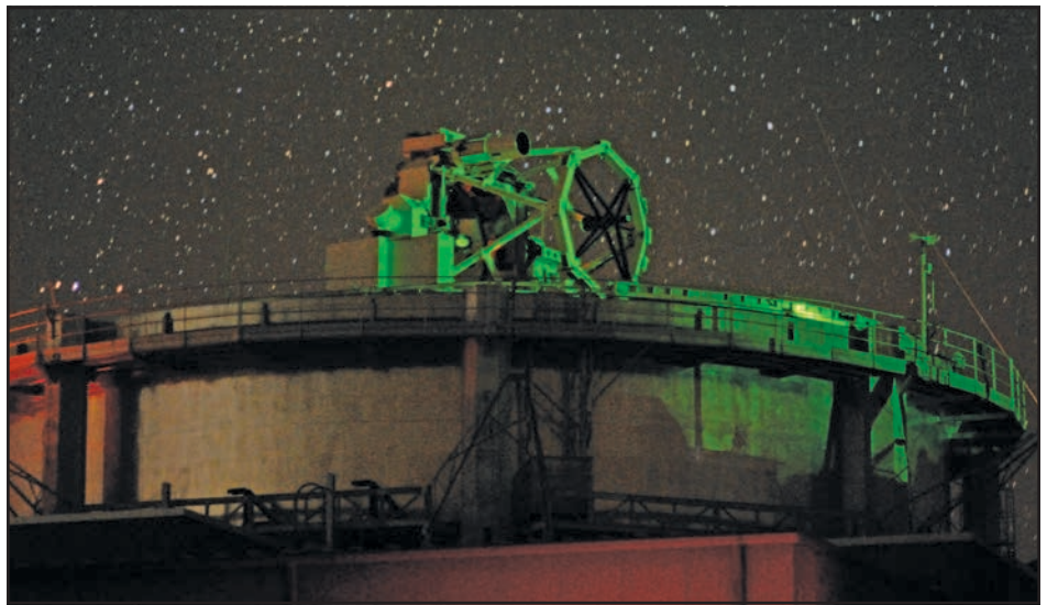
Air Force Research Laboratory's 3.6-meter, 75-ton Advanced Electro-Optical System (AEOS) telescope under laser illumination at its Directed Energy Directorate's (DED) Air Force Maui Optical and Surveillance Site, Maui, Hawaii. The illumination resulted from the multi-wave length laser propagation experiments that were completed at over 10,000 feet and over a 90-mile path between Mauna Loa on the island of Hawaii and the Air Force site atop the extinct volcano, Haleakala, on Maui. The DED is a mission of AEDC. (U.S. Air Force Photo by Rob Ratkowski)
