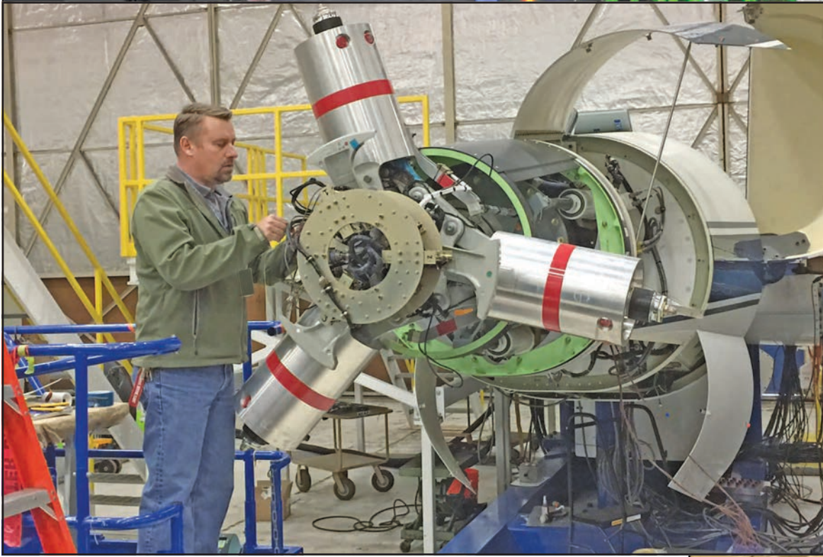
AEDC instrumentation engineer Dan Pruyn works on the Tiltrotor Test Rig in preparation for a test in the 40-foot by-80-foot wind tunnel at the National Full-Scale Aerodynamics Complex, the AEDC wind tunnel testing site located in California. The test of the TTR was a project sponsored by the National Aeronautics and Space Administration. TTR is a horizontal axis rig and rotates on the test section turntable to face the rotor into the wind at high speed, or fly edge-wise at low speed (100 knots), or at any angle in between. It is designed to accommodate a variety of rotors. (U.S. Air Force photo/Jeffrey Johnson)
